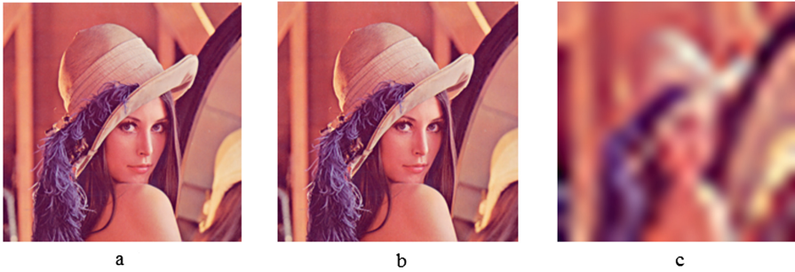
Fig. 4. Test image “Lena”: a - original image, 768 kB; b - high quality result, 164 kB; c - low quality result, 3 kB.
