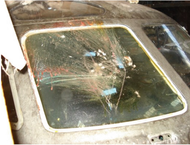
Fig. 5. Laminated windshield after testing.
